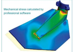
• Propeller mechanical analysis
