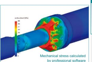
· Mechanical analysis of shaft joint
